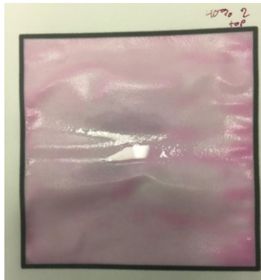
Figure 2.3: 5 mL sample of centrifuged solution is poured onto a 5 in \times 5 in square chromatography paper to spread the eggs and any remaining soil for imaging.
